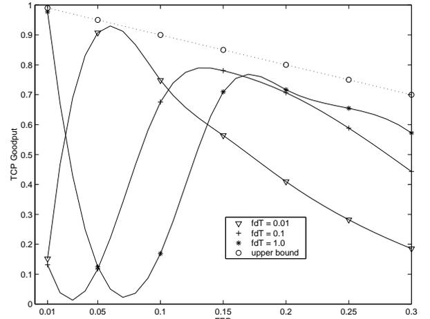
Figure 3: TCP goodput (awnd = 1024, data rate = 9600bps)
