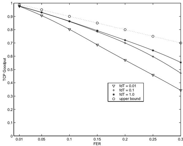
Figure 6: TCP goodput (awnd = 2, data rate = 9600bps)
