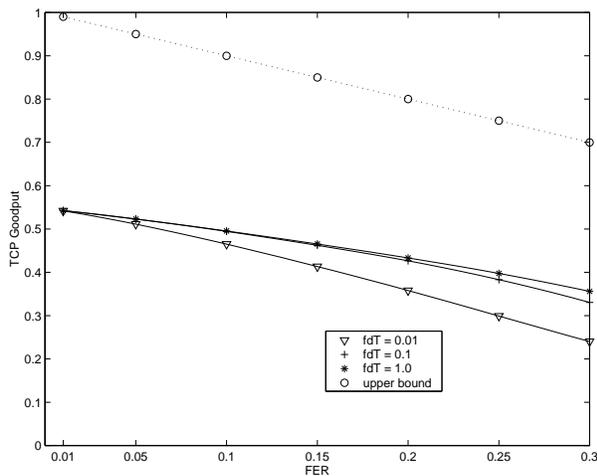
Figure 7: TCP goodput (awnd = 1, data rate = 9600bps)
