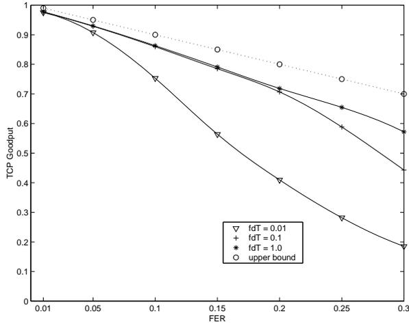
Figure 5: TCP goodput (awnd = 128, data rate = 9600bps)
