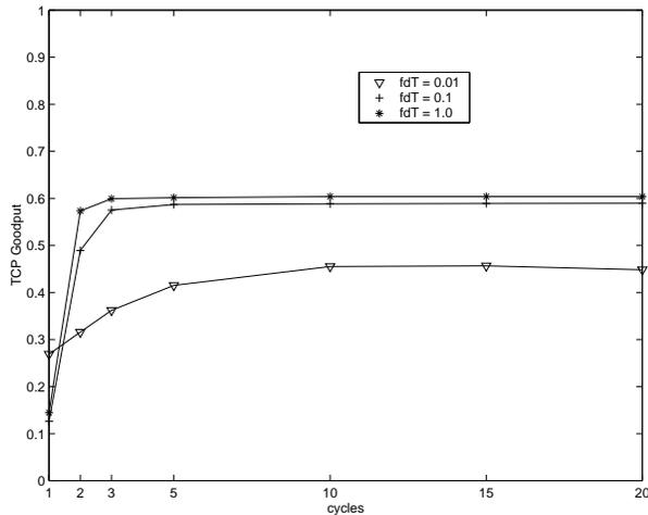
Figure 11: TCP goodput versus RLP retransmission cycles ( $P_e = 0.3$ )
