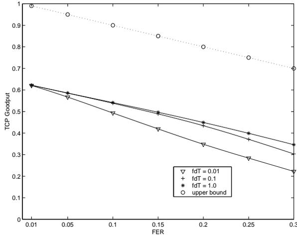
Figure 10: TCP goodput (awnd = 8, data rate = 16 × 9600bps)
