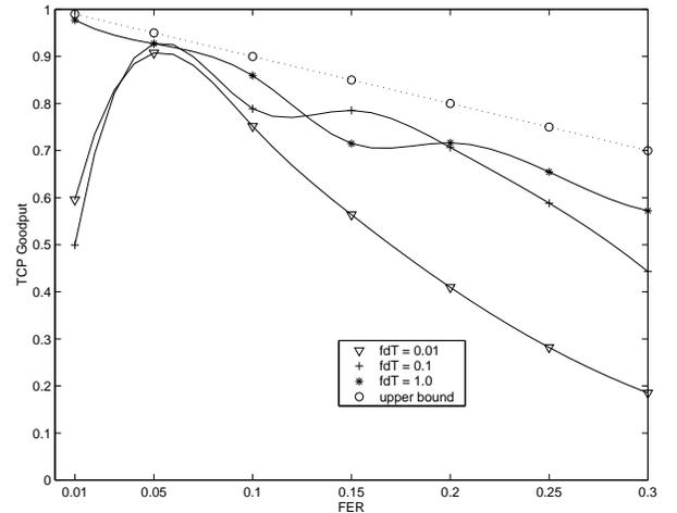
Figure 4: TCP goodput (awnd = 256, data rate = 9600bps)
