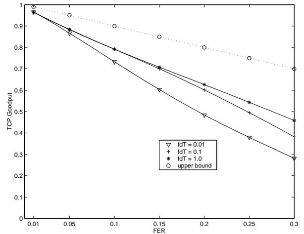
Figure 9: TCP goodput (awnd = 14, data rate = 16 × 9600bps)
