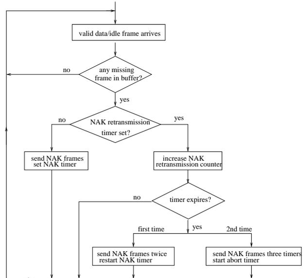
Figure 1: RLP one-cycle retransmissions
