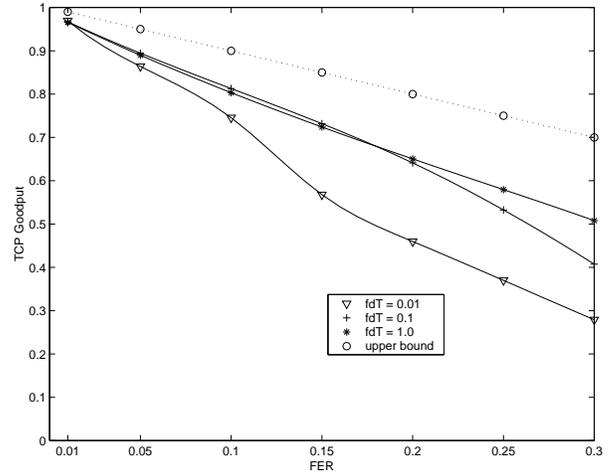
Figure 8: TCP goodput (awnd = 1024, data rate = 16 × 9600bps)
